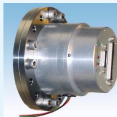
Open MCP Detector with fiber-coupled camera
