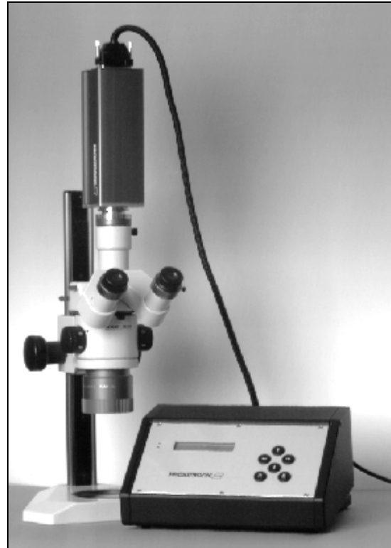
HL low light camera with Digital Control Unit connected to a microscope.
