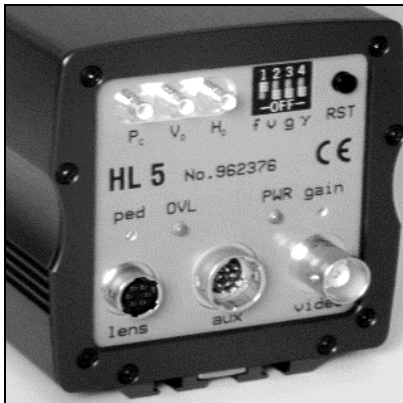
Rear view of HL5 low light camera with standard connectors and optional output signals PC, VD and HD.
